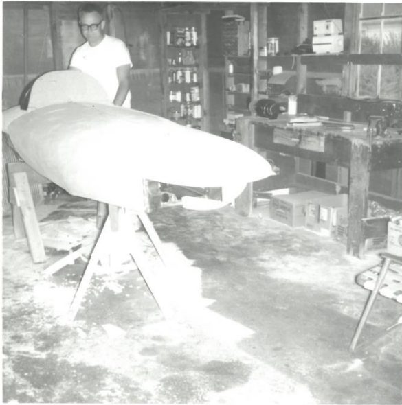
Body Buck of Plywood and Foam Built Over Tube Frame
