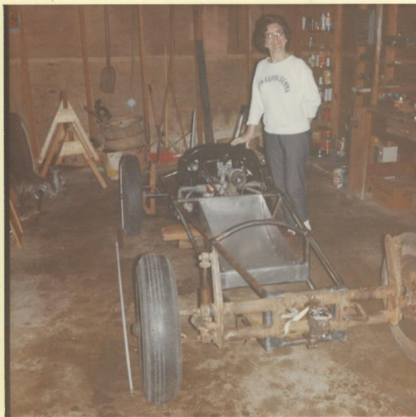
Chassis with Volkswagen Suspension and Engine
