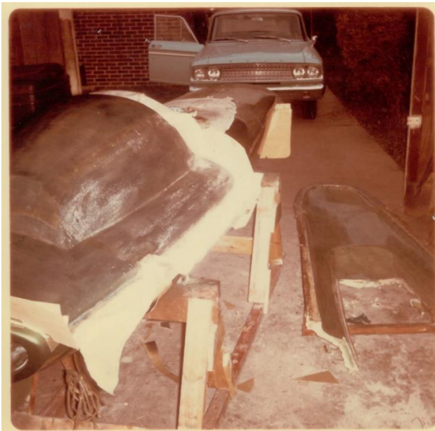
Tail Mold of Fiberglass Cloth and Polyester Resin
